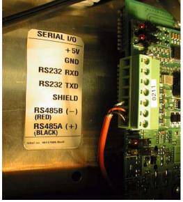
Connect to the serial I/O terminal block on the controller board.
