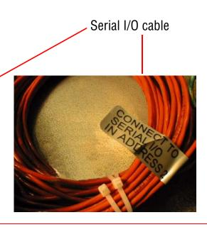
Run the serial I/O cable out of the first Master Unit through the communications conduit opening and close the sign.
