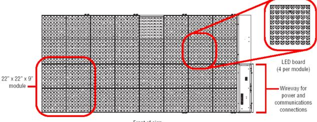
Front of sign Size: 2 module rows x 4 module columns
