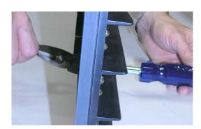
• Remove the screw with a phillips screwdriver.
