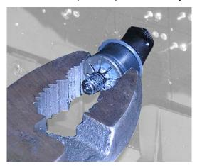
• Hold the retainer clip in place with pliers.
