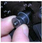
• On the other side of the driver board, slide the shim washer onto the screw.
