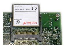
Although you can't see the back of the controller board, the compact flash card should slide in the grooves on the back. You may need to adjust the position of the flash card until you feel it slide in between the grooves.
