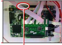
With the white label on the compact flash card facing the back of the sign, slide the flash card into the back of the controller board.
