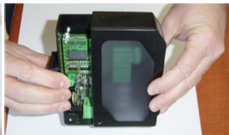
Slide the internal assembly out
