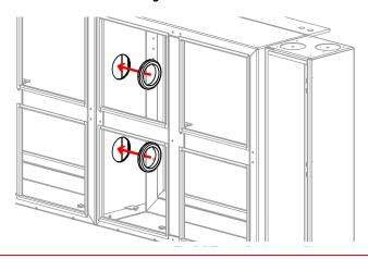
Connect the cables that are between each sign section:
