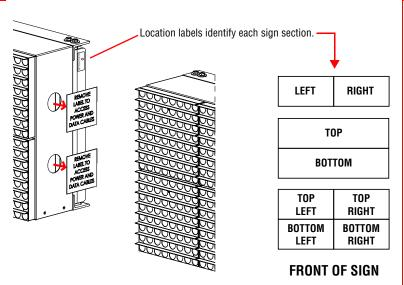
Mount sections flush with one another so that rubber grommets can be attached later (see step 4). Before continuing, make sure power has been removed from the sign.
