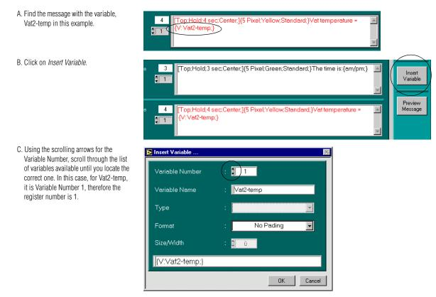
2. Set up a message instruction in the ladder logic to send the value of a variable to update a message in the sign.
