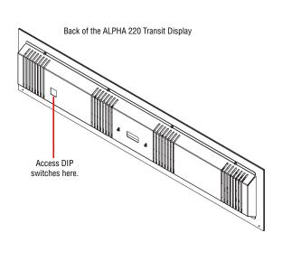
5. Plug the male DB25 connector from the RS232/RS485 Converter (train wiring) into the female DB25 connector at the display.
