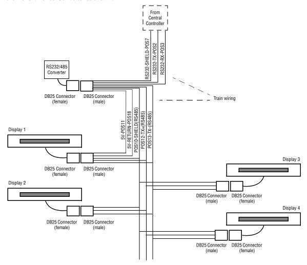
3. Connect the communications (RS485) wires from the male DB25 connector at the RS232/RS485 Converter (train wiring) to the male DB25 connector at each sign.
