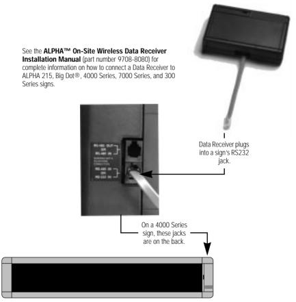
Figure 1: How to connect a Data Receiver to a sign.
