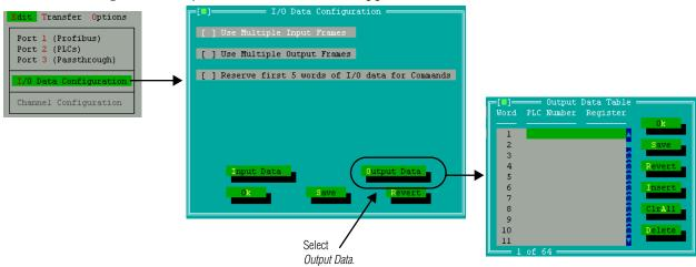
17. In the *Output Data Table*, you can press **Return** for the specific *Word* to use, or you can double click on that line. Then check the box to see the entries for that *Word*.
