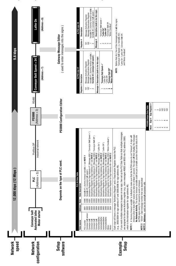
4. The complete setup for the PLC, PD3000, and ALPHA signs looks like this:
