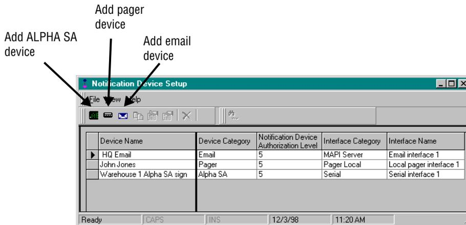
2. For this example, we will add an ALPHA SA sign with a direct serial interface connection, as shown here. See the table below for explanations.
