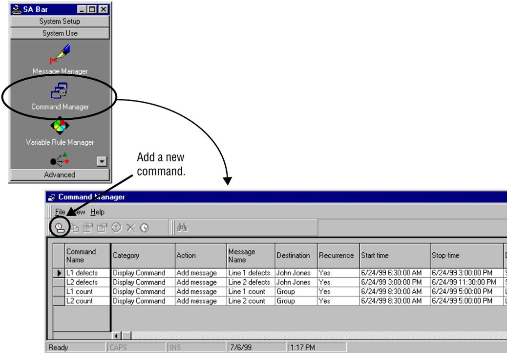
14. By either typing or using the drop-down arrows to select from a list, fill in the information as shown below for the Line 1 production count on the Line 1 sign. Click the *Destination* button to bring up a list, and select a *Destination* by clicking on the Line 1 *Destination* and then on the double-arrow button. Then click *OK*. Leave the start and end dates as they show on your screen and also the start time, but specify end time as three minutes from your current time. See below.
