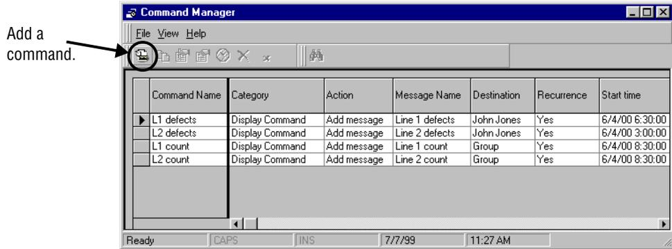
2. This example creates a command to add the message for the Line 1 production count on the Line 1 sign. The table below and the next steps explain each item and how to create it.
