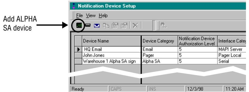
6. Fill in a name and description as desired. Specify the serial address of the sign. Choose "Serial Interface 1" for the *Interface Name*. Click the *Add* button.
