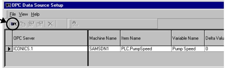
2. For this example, we will add a link to specific pump speed data coming from an OPC server on a networked computer. See the table below for explanations.
