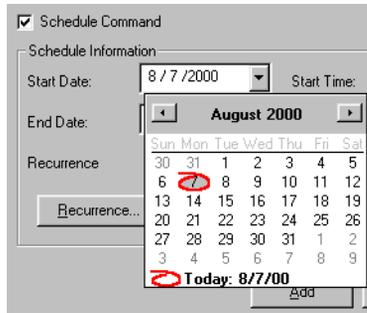
12. Complete the scheduling by setting the *Start* and *End Time*. Do this by clicking on each element of each time (that is, the hour, minute, or second) and then using the up- or down-arrows to increase or decrease the setting. You can also type the number.
