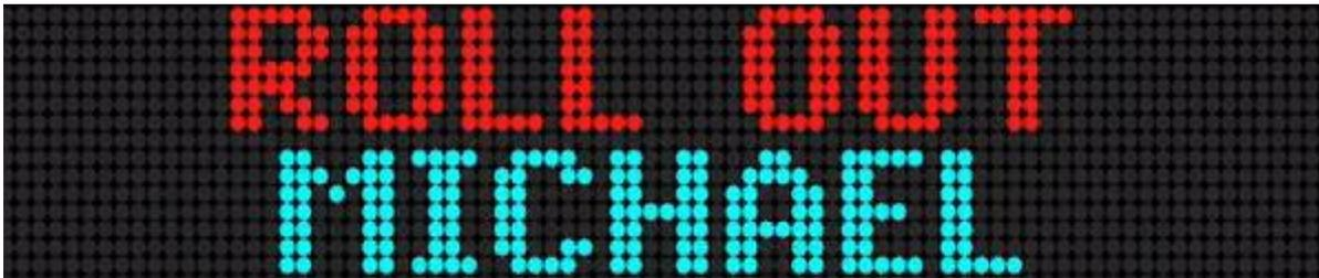
Roll Out Mode using 7-Pixel Characters on a Two-Line Sign
