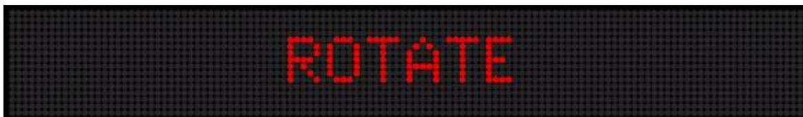
Rotate Mode using 16-Pixel Characters on a Two-Line Sign
