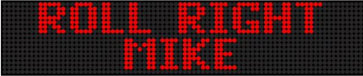
Roll Right Mode using 7-Pixel Characters on a Two-Line Sign
