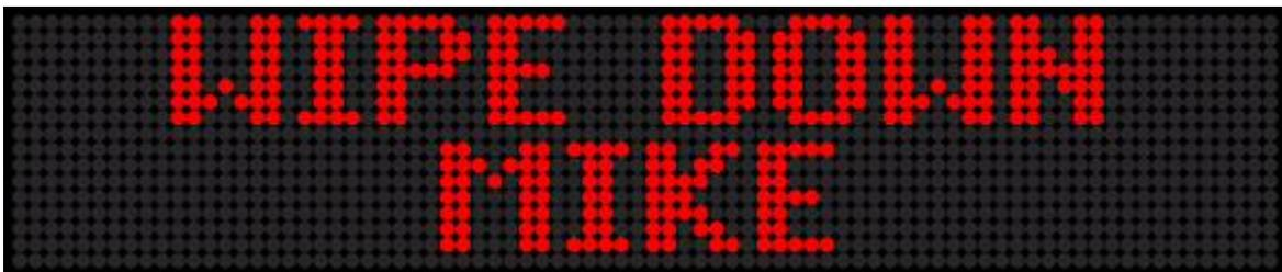
Wipe Down Mode using 7-Pixel Characters on a Two-Line Sign
