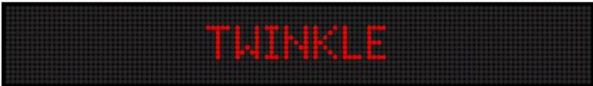
Twinkle Mode using 16-Pixel Characters on a Two-Line Sign
