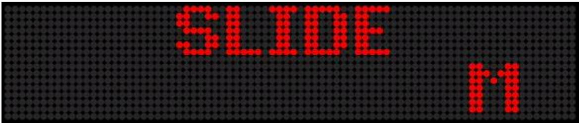
Slide Mode using 7-Pixel Characters on a Two-Line Sign
