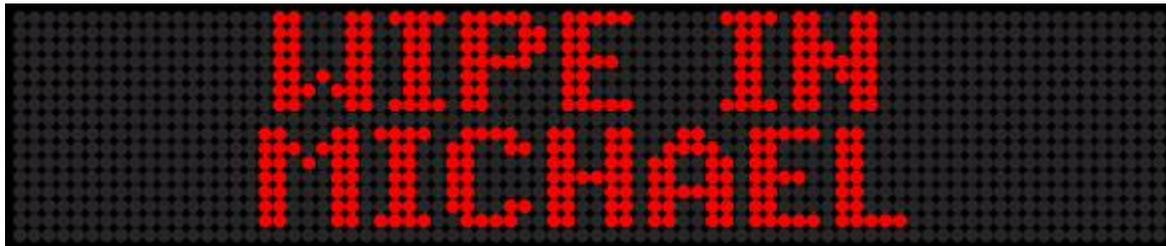
Wipe In Mode using 7-Pixel Characters on a Two-Line Sign
