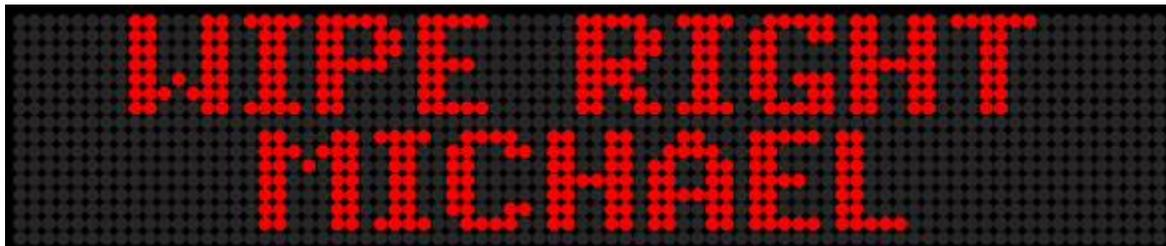
Wipe Right Mode using 7-Pixel Characters on a Two-Line Sign
