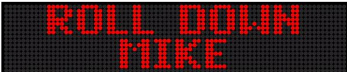
Roll Down Mode using 7-Pixel Characters on a Two-Line Sign
