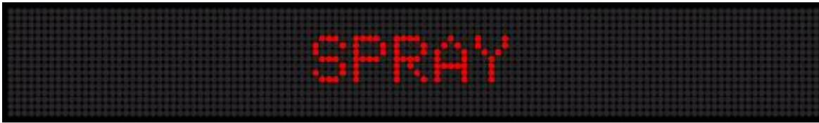
Spray Mode using 16-Pixel Characters on a Two-Line Sign
