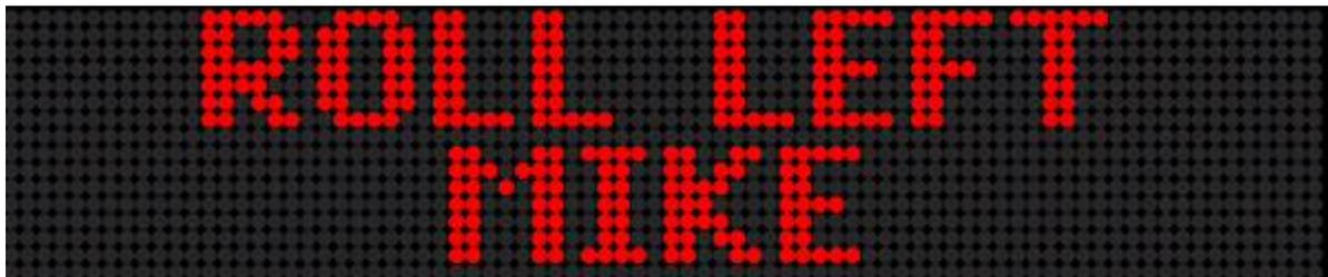
Roll Left Mode using 7-Pixel Characters on a Two-Line Sign
