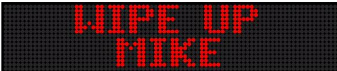
Wipe Up Mode using 7-Pixel Characters on a Two-Line Sign
