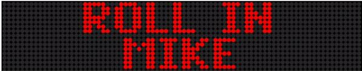
Roll In Mode using 7-Pixel Characters on a Two-Line Sign
