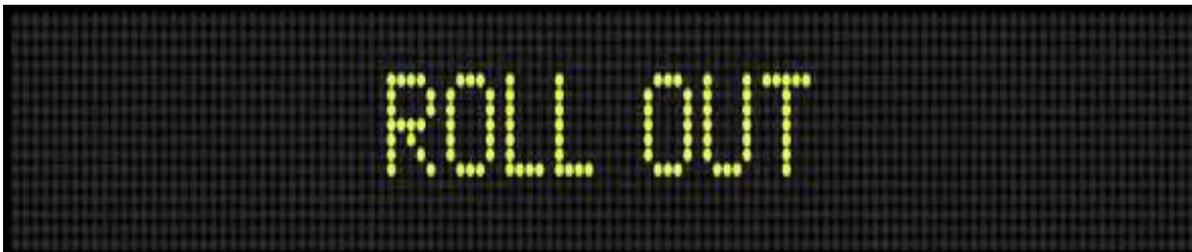
Roll Out Mode using 16-Pixel Characters on a Two-Line Sign
