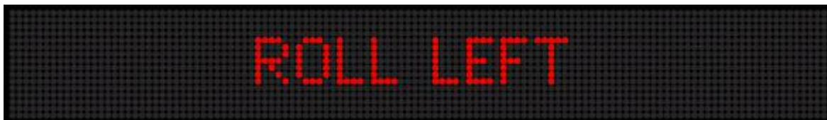
Roll Left Mode using 16-Pixel Characters on a Two-Line Sign
