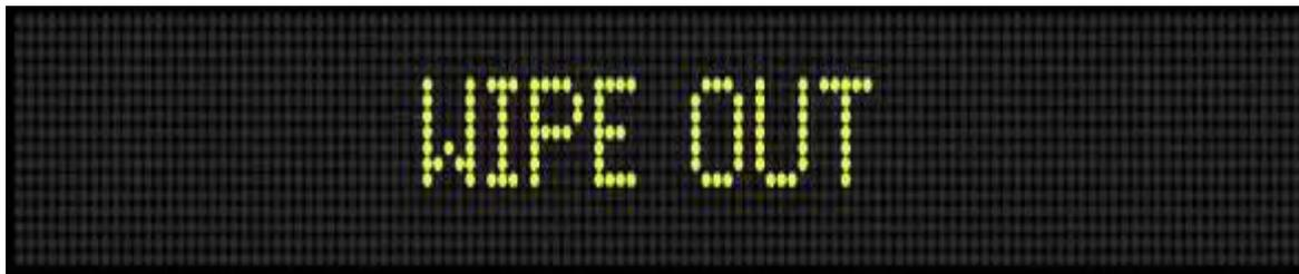
Wipe Out Mode using 16-Pixel Characters on a Two-Line Sign
