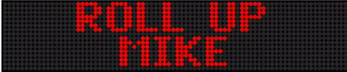
Roll Up Mode using 7-Pixel Characters on a Two-Line Sign
