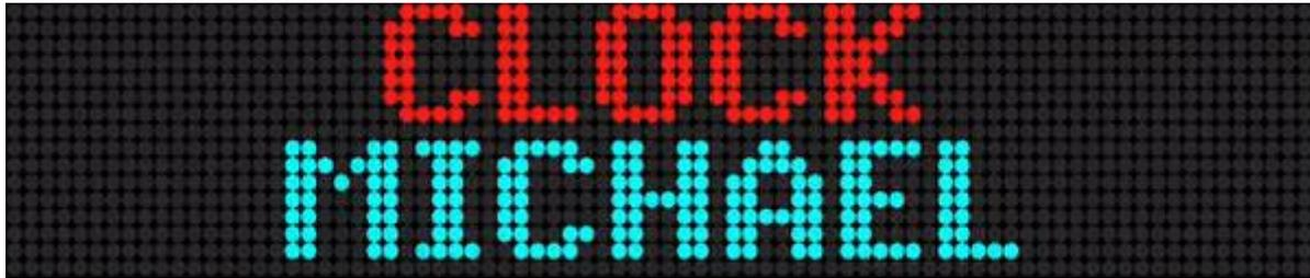
Clock Mode using 7-Pixel Characters on an RGB Two-Line Sign
