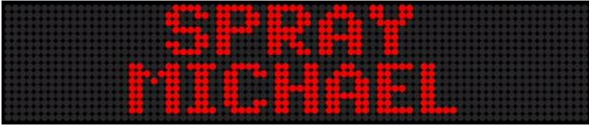
Spray Mode using 7-Pixel Characters on a Two-Line Sign
