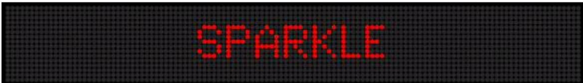
Sparkle Mode using 16-Pixel Characters on a Two-Line Sign
