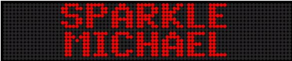
Sparkle Mode using 7-Pixel Characters on a Two-Line Sign
