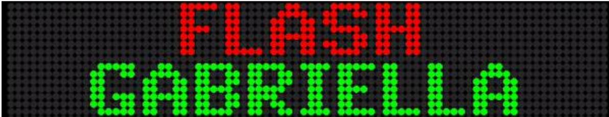
Flash Mode using 7-Pixel Characters on a Two-Line Sign
