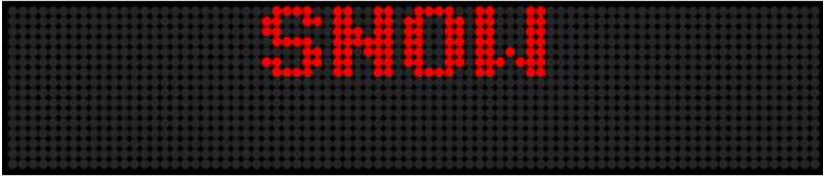
Snow Mode using 7-Pixel Characters on a Two-Line Sign
