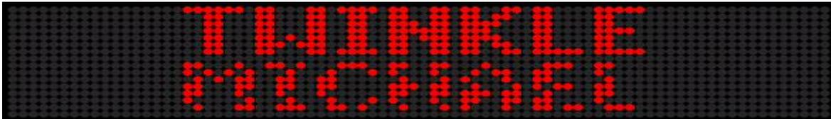
Twinkle Mode using 7-pixel Characters on a Two-Line Sign
