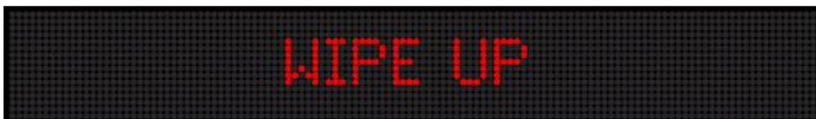
Wipe Up Mode using 16-Pixel Characters on a Two-Line Sign
