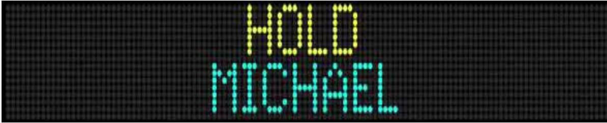
Hold Mode using 7-Pixel Characters on a Two-Line Sign
