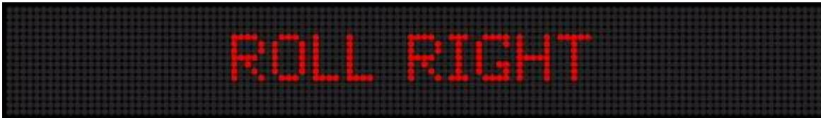
Roll Right Mode using 16-Pixel Characters on a Two-Line Sign
