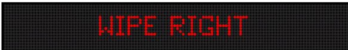
Wipe Right Mode using 16-Pixel Characters on a Two-Line Sign
