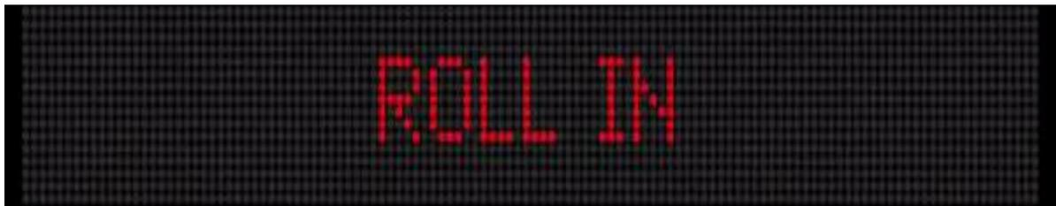
Roll In Mode using 16-Pixel Characters on a Two-Line Sign
