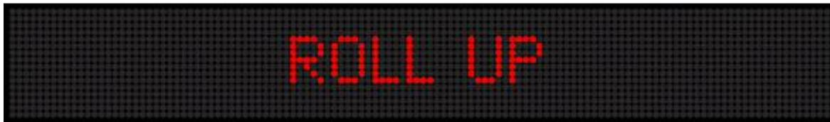
Roll Up Mode using 16-Pixel Characters on a Two-Line Sign
