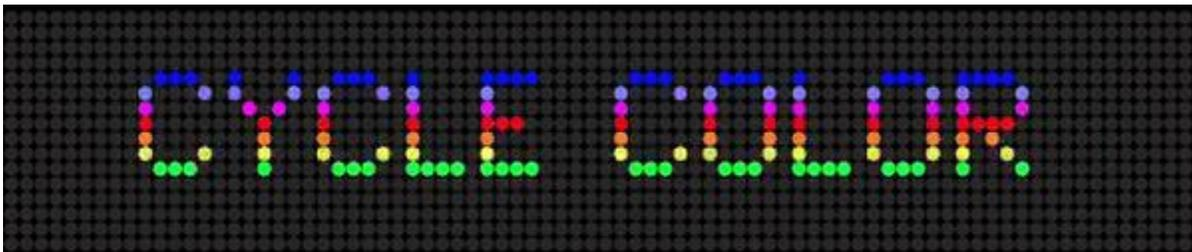
Cycle Color Mode using 16-Pixel Characters on an RGB Two-Line Sign
