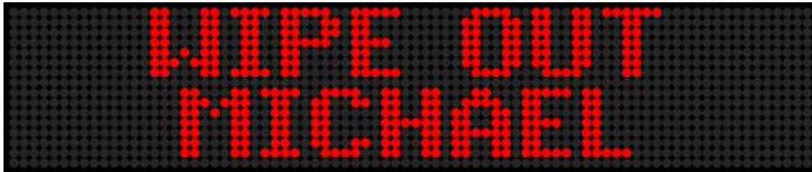
Wipe Out Mode using 7-Pixel Characters on a Two-Line Sign
