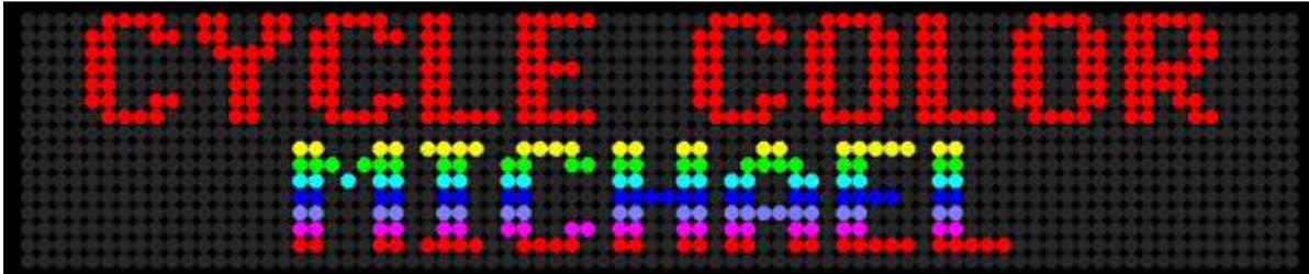
Cycle Color Mode using 7-Pixel Characters on an RGB Two-Line Sign
