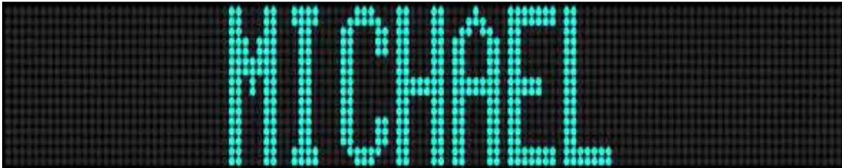
Hold Mode using 16-Pixel Characters on a Two-Line Sign
