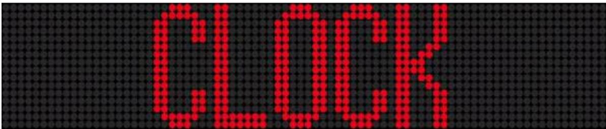
Clock Mode using 16-Pixel Characters on an RGB Two-Line Sign
