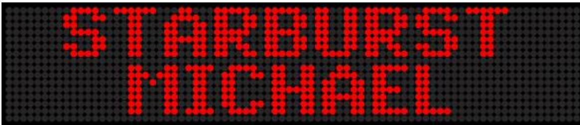
Starburst Mode using 7-Pixel Characters on a Two-Line Sign
