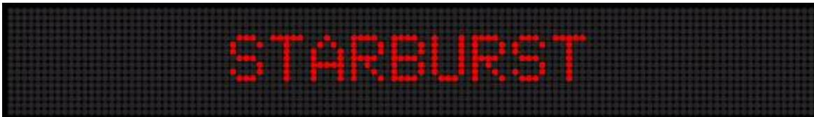
Starburst Mode using 16-pixel Characters on a Two-Line Sign
