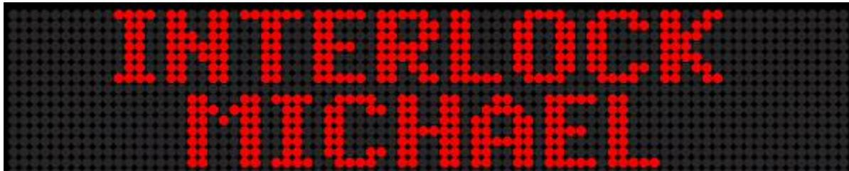
Interlock Mode using 7-Pixel Characters on a Two-Line Sign
