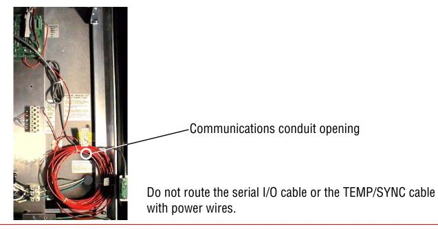
**Open the sign labeled SLAVE UNIT, SERIAL ADDRESS = 2 and run the serial I/O** cable and the TEMP/SYNC cable into the sign through the communications conduit opening.
