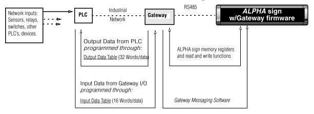
INFORMATION FLOW—In a Profibus DP network, a "device" is any point in the information pathway that is capable of sending or receiving a data signal. In the most basic network configuration, above (one input, one PLC, one Gateway interface, one sign), the PLC, Gateway interface, and sign are all capable of both sending and receiving data signals.
