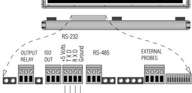
3. Cut off the jack from the end of the RS-232 cable that has the ferrite protector.
