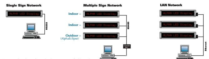
\*The RS485 converter box, Ethernet Adapter and wireless components are all sold separately.
